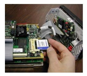
18. \_\_\_\_ Remove CompactFlash.
