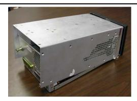
11. \_\_\_\_\_ Slide cover back – front end may "stick" for first half-inch of travel.
