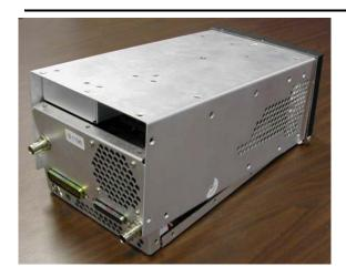
25. \_\_\_\_ Squeeze front end of cover into bezel. It may be slightly stiff.
