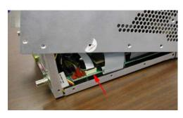
12. \_\_\_\_ Lift rear of cover to reveal white Flex-Cable.
