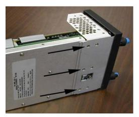
16. \_\_\_\_ Remove the 3 rear-most #4-40 Flathead Screws from bottom of Display Assembly which connects the cover to the chassis.
