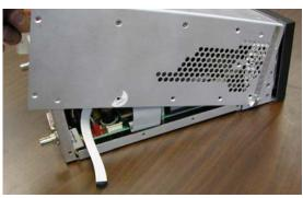
23. Position cover in place, holding the rear end up.
