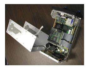
15. \_\_\_\_\_ Set cover aside. There is no need to remove the coax
