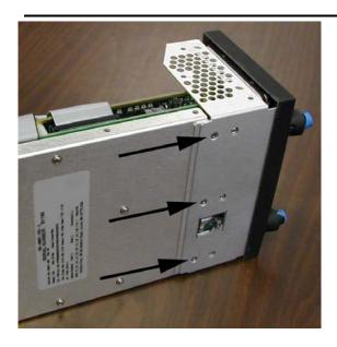
22. \_\_\_\_\_ Re-assemble Display Assembly with 3x #4-40 Flathead Screws.
