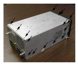
26. \_\_\_\_ Re-assemble cover with 24x #4-40 Flathead Screws and 3x black #4-40 Flathead Screws.
