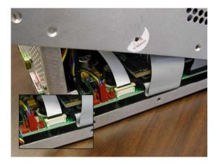
24. \_\_\_\_\_ Insert white Flex-Cable into ZIF connector. Make certain it is inserted until the cable hits the stop. Push top of ZIF connector down.
