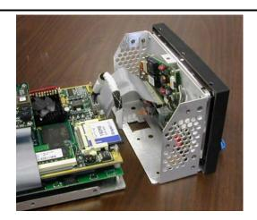
17. \_\_\_\_\_ Slide Display Assembly forward.
