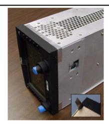
8. Peel back aluminum tape from the bottom of the unit. Leave attached to the cover.
