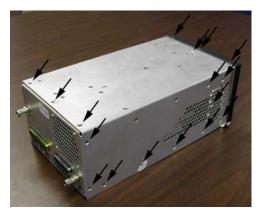
9. \_\_\_\_ Remove the 24x #4-40 Flathead Screws, and 3x black #4-40 Flathead Screws. Note that the Warranty-Voided stickers will need to be broken.
