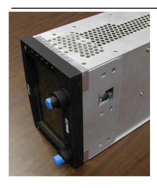
27. \_\_\_\_ Re-apply aluminum tape as shown.
